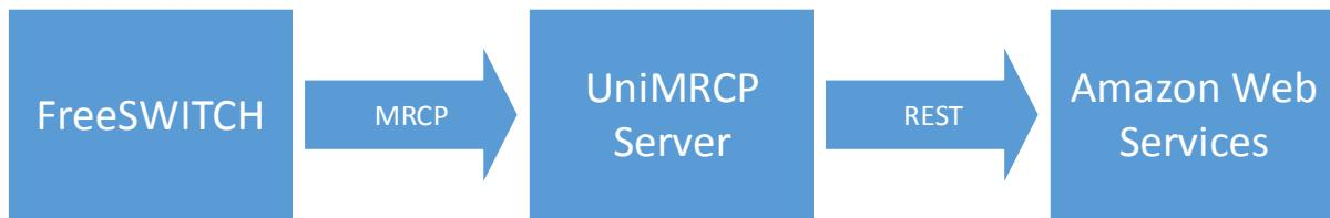
Note that the FreeSWITCH and the UniMRCP server typically reside on different hosts in a LAN, although both might be installed on the same host.
