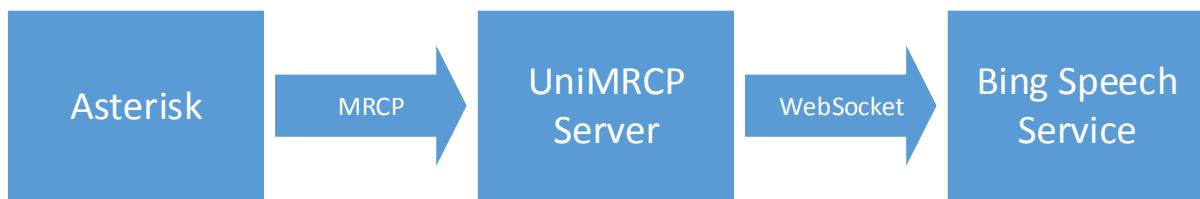
Note that the Asterisk and the UniMRCP server typically reside on different hosts in a LAN, although both might be installed on the same host.
